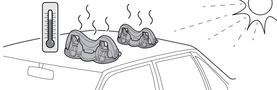
**US** Do not leave the carrier mounted on the roof in temperatures exceeding 30 °C (86 °F). Such excessive temperatures may cause the magnetic pad to lose its ability to adhere to the roof or cause damage to the car's paint.
