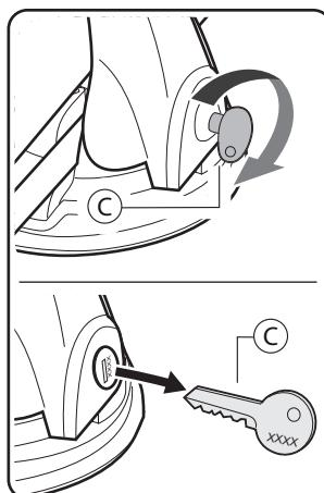
**US** Close the clamp to secure the cargo. Failure to close the clamp properly will result in the load falling off. Turn the key clockwise to lock the carrier. NB. Make sure to remove the key before driving.
