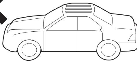
**US** This magnetic carrier should be installed only on smooth roofs, without features such as sun roofs, T-tops, targa tops, ribs, luggage racks, etc. The carrier should be installed on a flat area, so as to avoid the ribs if your car has them.
