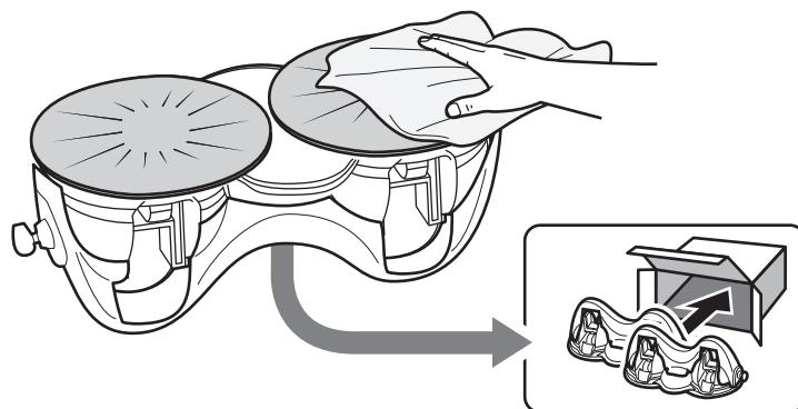
**US** Wash any mud off of the carrier system. Use only a mild detergent to clean the carrier, if necessary. Use a damp cloth to wipe away dust and dirt. You may use the original box to store your carrier when not in use.
