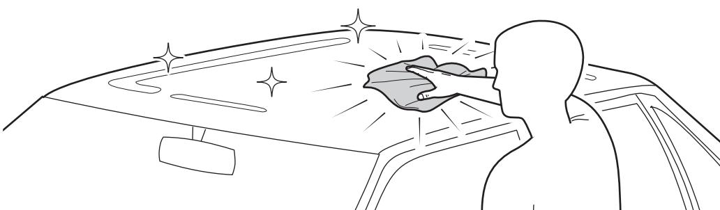
**US** This carrier is designed to be mounted on the car roof using magnetic power. It is important to keep the roof surface clean and free from any contaminants that could come between the carrier and the roof while driving.
