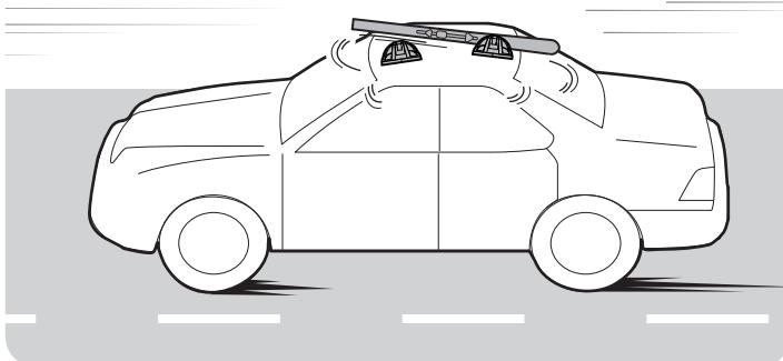
**US** After driving continuously for some time, check to see that the carrier and cargo are still securely mounted.
