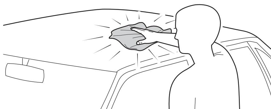
**US** Before installing your carrier, clean the surface of your vehicle's roof and the magnetic sheets.
