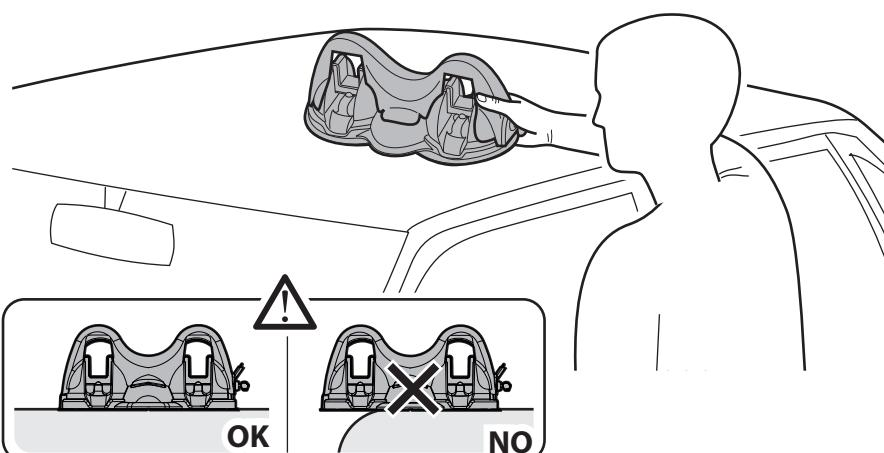
**US** Determine the installation position. When on the roof, the entire magnetic pad must be in contact with the roof.
