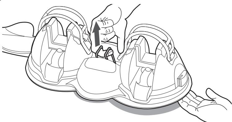
**US** To remove the carrier, pull the hook upward to break the magnetic seal.
