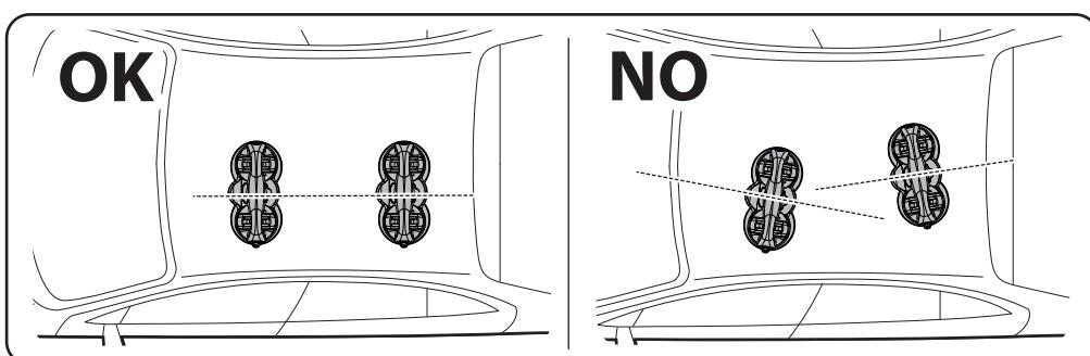
**US** The front and rear carriers must be installed parallel to each other.
