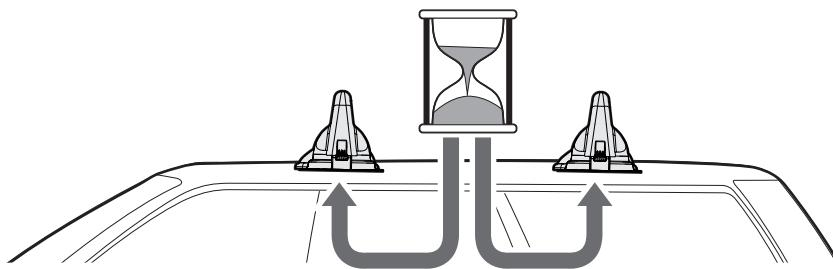
**US** Never leave the carrier mounted on the roof for longer than 36 hours at a time. Otherwise, the magnetic pad may lose its ability to adhere to the roof or damage the car's paint.
